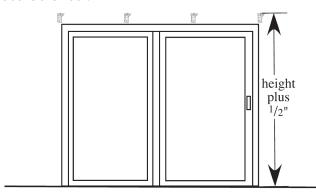
The two brackets on the end should be positioned within 4" of the end of the track. Space additional brackets evenly. Mount all brackets level at the same height.
