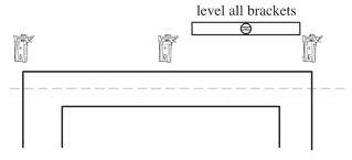
Be sure to also use all of the brackets provided. A level and well supported track will ensure smooth operation.
