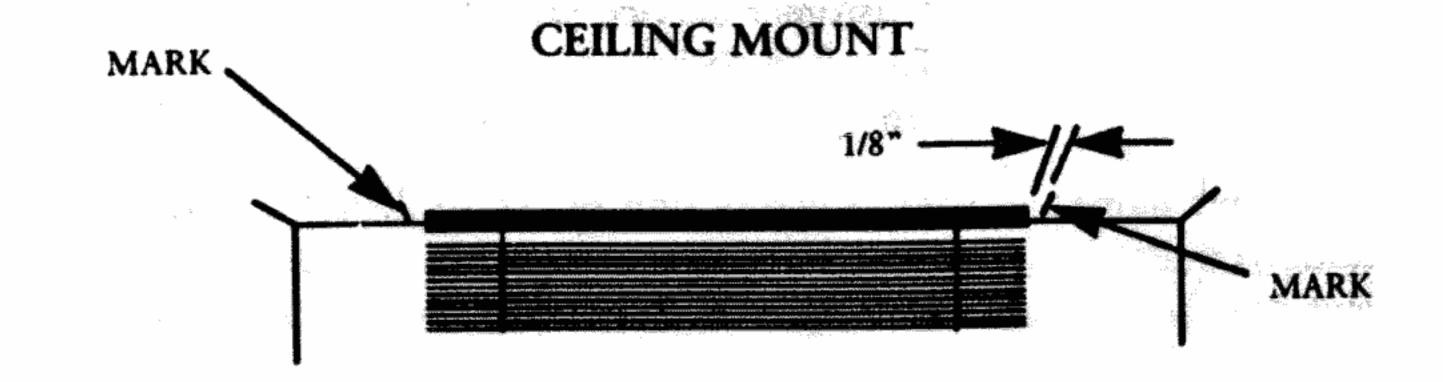
The end brackets may be mounted using two screws in several different orientations depending on your needs:
