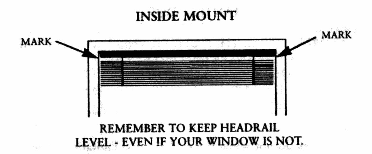
For a Ceiling or Overhead Mount, hold the blind against the ceiling centered in front of the window and make pencil marks 1/8" beyond the ends of the headrail. The right and left installation brackets will be placed on these marks.
