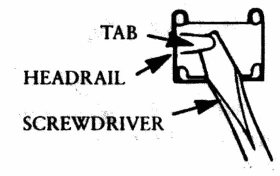
If your blind fits too tightly, press the tab(s) in with a pair of pliers. Now reinstall the headrail and close the mounting bracket covers.
