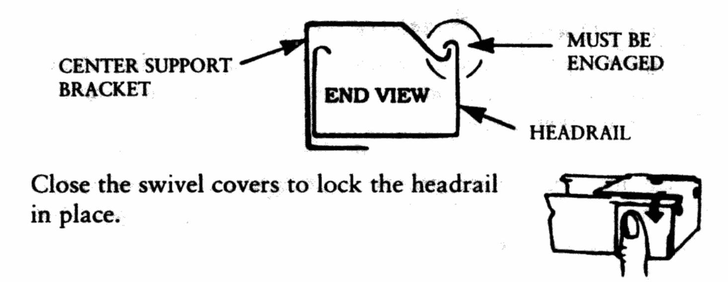
If your blind is not fitting snugly left to right, open the mounting brackets, remove the headrail and pry out the tab(s) at the ends of the headrail a bit with a screwdriver
