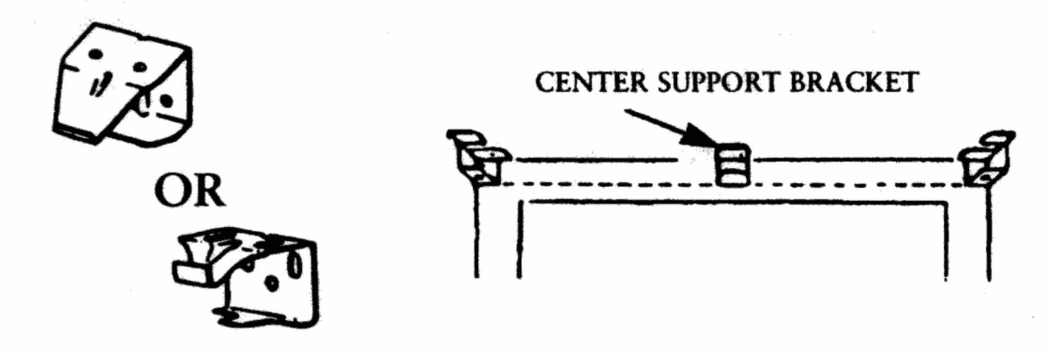
Snap the valance clips over the front lip of the headrail before mounting the blind to the installation brackets. A valance clip is furnished for every ladder. Install the valance clip next to each ladder. If the clips are mounted directly in line with the ladders, they may catch on the cords inside the headrail.
