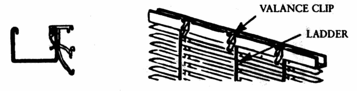
Insert the headran into the end brackets. If an auxiliary support bracket is used, be sure that it is properly engaged with headrail.
