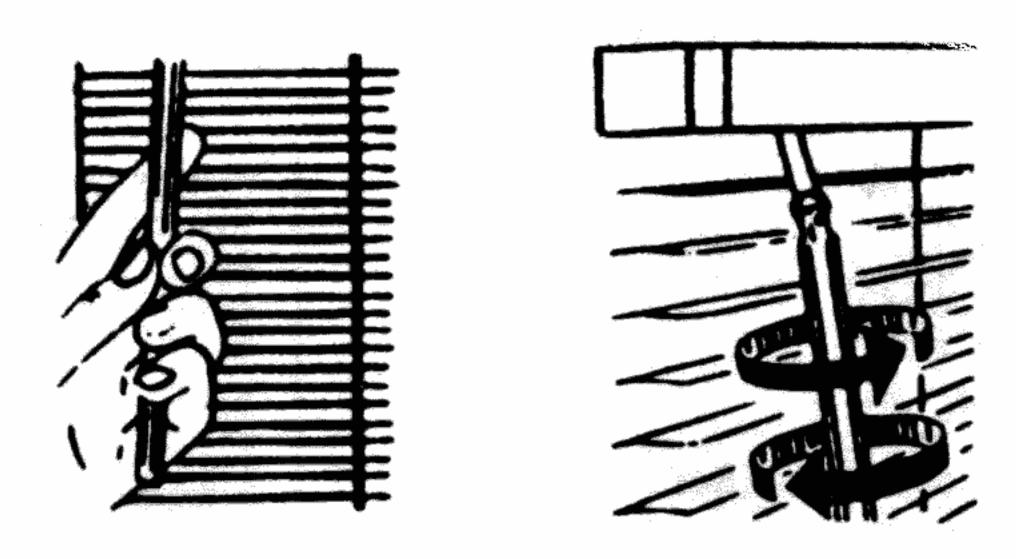
RAISE OR LOWER: Slats should be fully open, not tilted, when raising or lowering. To raise blind, pull lift cord straight down. To lower blind, pull cord toward center of blind and slowly raise your hand while holding onto the cord.
