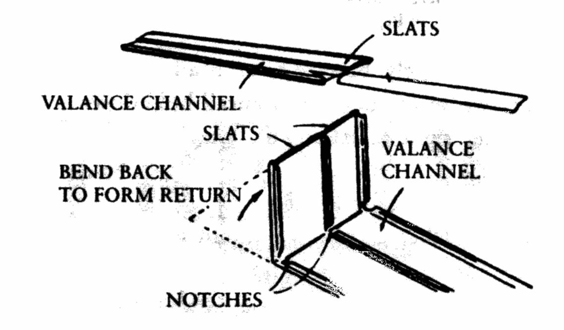
Starting at one end, place the upper lip of the valance into the top groove of the valance bracket. Carefully snap the lower lip into the bottom groove on the bracket. Repeat this at each bracket. Valance return length may be trimmed with scissors if necessary.
