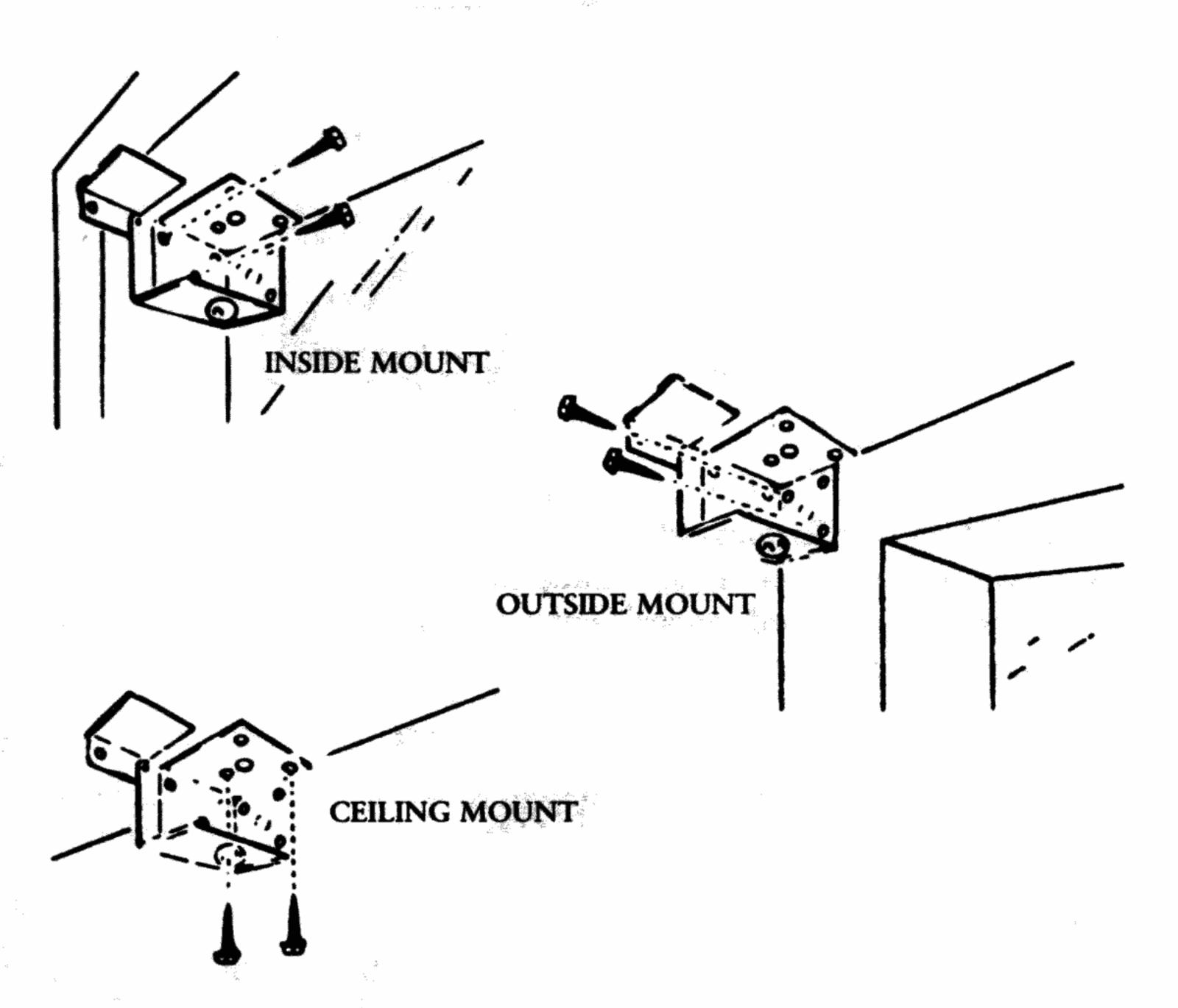
Use proper screws. Two screws are supplied for each mounting bracket. These are suitable for most wood and sheet metal surfaces. On wood surfaces pre-drill homes for the screws using a 1/16" dia. drill bit or make a starter hole with a finishing nail and hammer or awl. On sheet metal surfaces use a 3/32" dia. steel drill bit. For plaster, drywall, concrete, stone, brick or tile use appropriate plugs, anchors or screws of the proper type and length. Follow the manufacturers recommendations.
